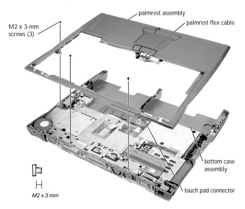
8 Using the plastic scribe along the edge of the plastic, remove the palmrest assembly from the bottom case assembly.
