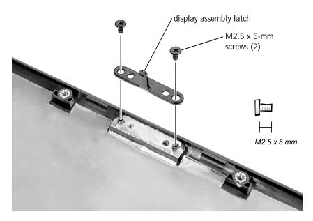
Removing the Display Assembly Latch
